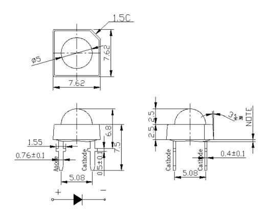
Units: mm / tolerance = +/-0.2mm
