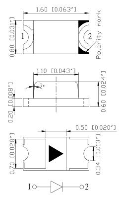
Units: mm / tolerance = +/-0.1mm
