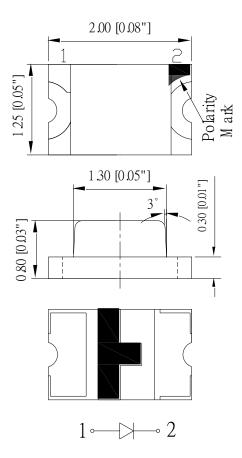
Units: mm / tolerance = +/-0.1mm
